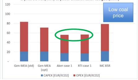
Avoided cost incl. power CO2 footprint (Coal price 400 NOK/ton and El price 0.4 NOK/kWh; El. power emission factor 131 gCO2/kWh)
